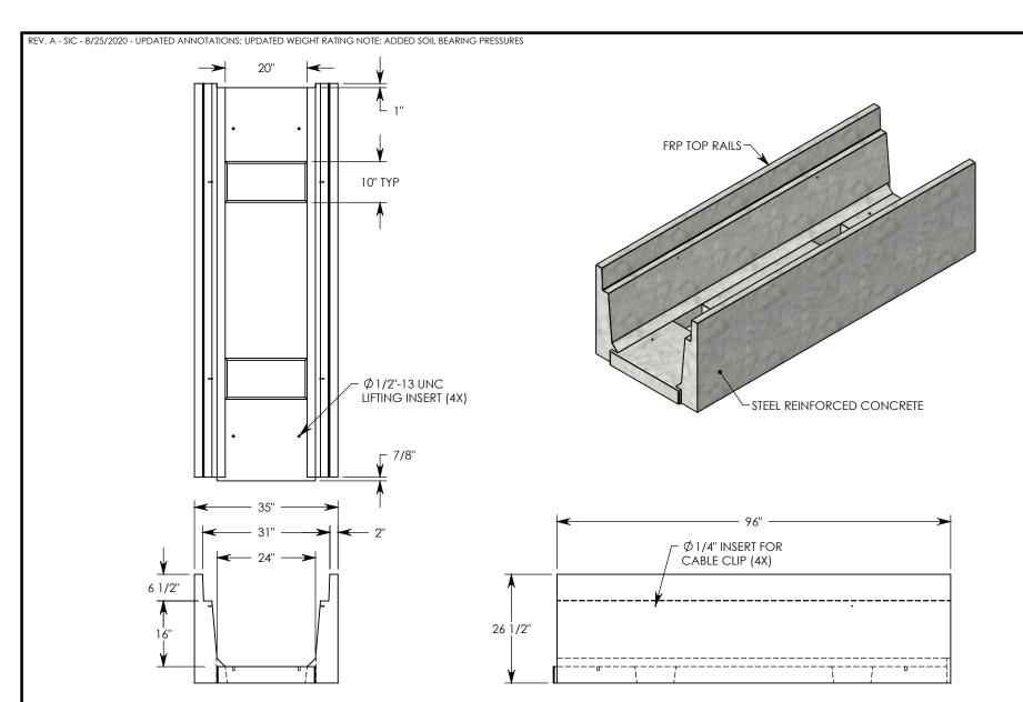
**NOTE 1:** FOR NON-STANDARD LENGTHS THE CHANNEL WILL BE SOLID BOTTOM AND DESIGNATED WITH ITS CORRESPONDING LENGTH MEASUREMENT. IE: HT6F2416 32"
