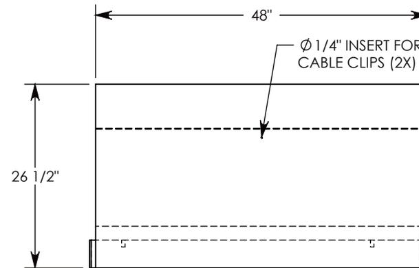
**NOTE 1:** FOR NON-STANDARD LENGTHS THE CHANNEL WILL BE SOLID BOTTOM AND DESIGNATED WITH ITS CORRESPONDING LENGTH MEASUREMENT. IE: HT6F2416 36"
