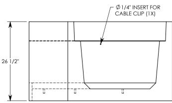
MAX AASHTO H-40 RATED - 64,000 LB. SINGLE AXLE LOAD DEPENDENT ON TRENCH COVER RATING MINIMUM ALLOWABLE SOIL BEARING PRESSURE – H-40: 3,500 PSF; H-20: 3,000 PSF
