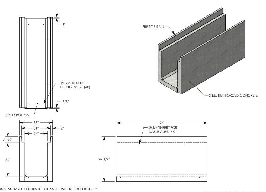
**NOTE 1:** FOR NON-STANDARD LENGTHS THE CHANNEL WILL BE SOLID BOTTOM AND DESIGNATED WITH ITS CORRESPONDING LENGTH MEASUREMENT. IE: HT6F2436 36"
