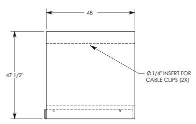
**NOTE 1:** FOR NON-STANDARD LENGTHS THE CHANNEL WILL BE SOLID BOTTOM AND DESIGNATED WITH ITS CORRESPONDING LENGTH MEASUREMENT. IE: HT6F2436 36"
