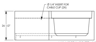
MAX AASHTO H-40 RATED - 64,000 LB. SINGLE AXLE LOAD DEPENDENT ON TRENCH COVER RATING MINIMUM ALLOWABLE SOIL BEARING PRESSURE – H-40: 3,000 PSF; H-20: 3,000 PSF
