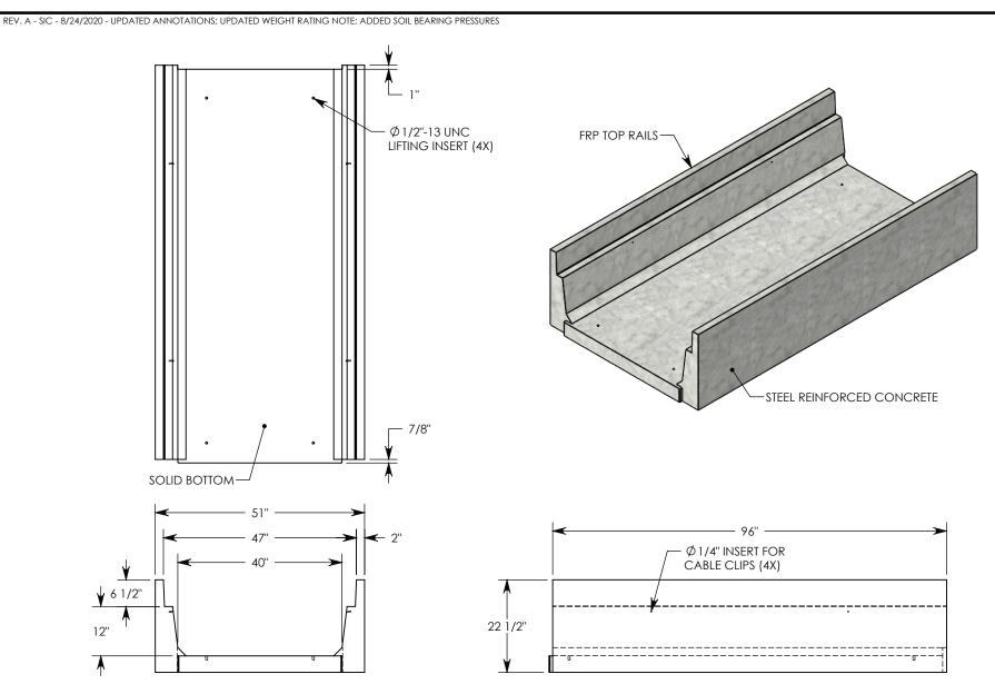
**NOTE 1:** FOR NON-STANDARD LENGTHS THE CHANNEL WILL BE SOLID BOTTOM AND DESIGNATED WITH ITS CORRESPONDING LENGTH MEASUREMENT. IE: HT6F4012 36"
