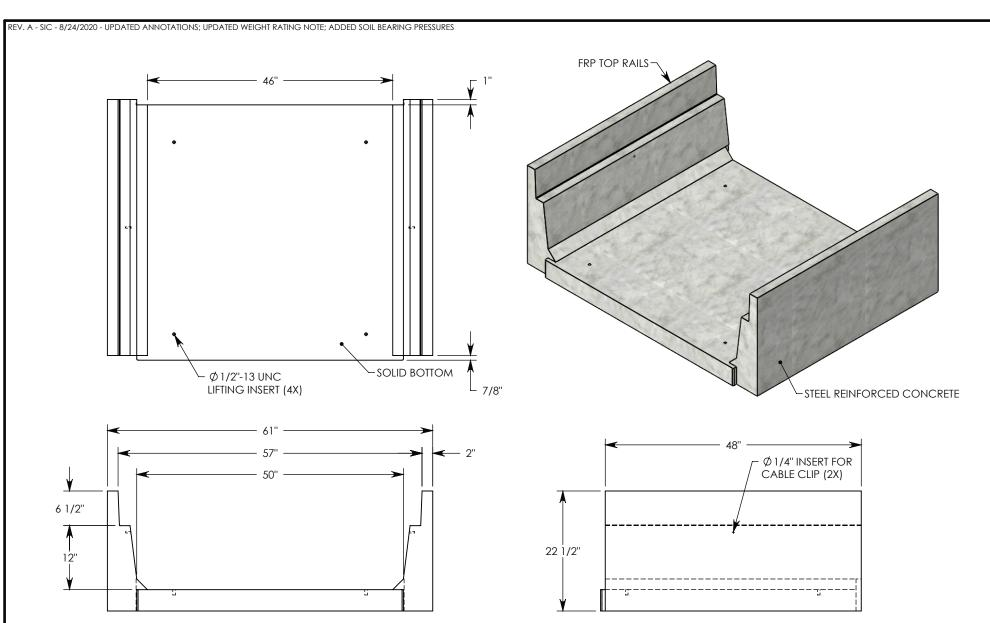
**NOTE 1:** FOR NON-STANDARD LENGTHS THE CHANNEL WILL BE SOLID BOTTOM AND DESIGNATED WITH ITS CORRESPONDING LENGTH MEASUREMENT. IE: HT6F5012 32"
