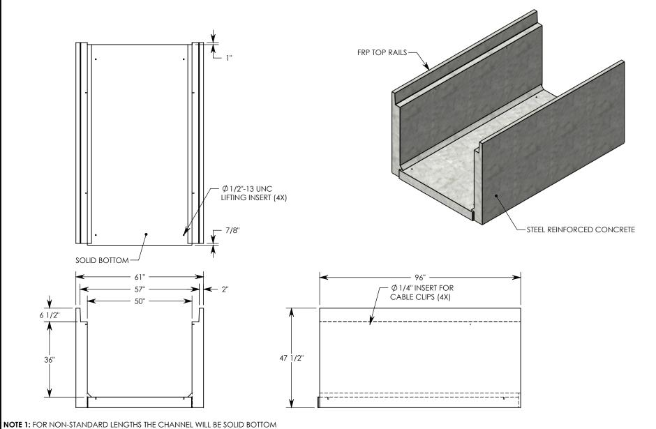
**NOTE 1:** FOR NON-STANDARD LENGTHS THE CHANNEL WILL BE SOLID BOTTOM AND DESIGNATED WITH ITS CORRESPONDING LENGTH MEASUREMENT. IE: HT6F5036 36"
