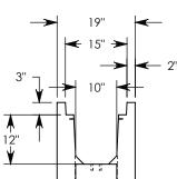
NOTE 1: FOR NON-STANDARD LENGTHS THE CHANNEL WILL BE SOLID BOTTOM AND DESIGNATED WITH ITS CORRESPONDING LENGTH MEASUREMENT. IE: HTF1012 32"
