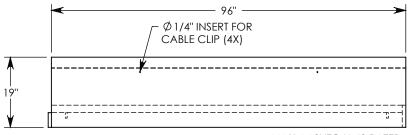
MAX AASHTO H-40 RATED - 64,000 LB. SINGLE AXLE LOAD DEPENDENT ON TRENCH COVER RATING MINIMUM ALLOWABLE SOIL BEARING PRESSURE – H-40: 5,000 PSF; H-20: 3,000 PSF
