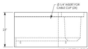
MAX AASHTO H-40 RATED - 64,000 LB. SINGLE AXLE LOAD DEPENDENT ON TRENCH COVER RATING MINIMUM ALLOWABLE SOIL BEARING PRESSURE – H-40: 5,500 PSF; H-20: 3,000 PSF
