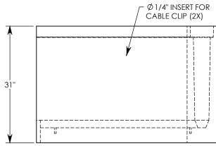
MAX AASHTO H-40 RATED - 64,000 LB. SINGLE AXLE LOAD DEPENDENT ON TRENCH COVER RATING MINIMUM ALLOWABLE SOIL BEARING PRESSURE – H-40: 5,500 PSF; H-20: 3,000 PSF
