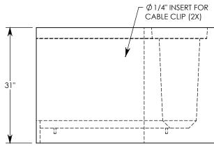
MAX AASHTO H-40 RATED - 64,000 LB. SINGLE AXLE LOAD DEPENDENT ON TRENCH COVER RATING MINIMUM ALLOWABLE SOIL BEARING PRESSURE – H-40: 5,500 PSF; H-20: 3,000 PSF
