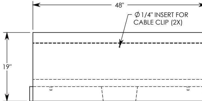
**NOTE 1:** FOR NON-STANDARD LENGTHS, THE CHANNEL WILL BE SOLID BOTTOM AND DESIGNATED WITH ITS CORRESPONDING LENGTH MEASUREMENT. IE: HTF2012 32"
