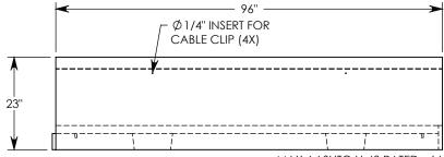
**NOTE 1:** FOR NON-STANDARD LENGTHS THE CHANNEL WILL BE SOLID BOTTOM AND DESIGNATED WITH ITS CORRESPONDING LENGTH MEASUREMENT. IE: HTF2016 32"
