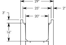
**NOTE 1:** FOR NON-STANDARD LENGTHS THE CHANNEL WILL BE SOLID BOTTOM AND DESIGNATED WITH ITS CORRESPONDING LENGTH MEASUREMENT. IE: HTF2016 72"
