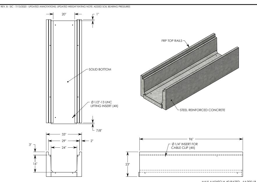
**NOTE 1:** FOR NON-STANDARD LENGTHS THE CHANNEL WILL BE SOLID BOTTOM AND DESIGNATED WITH ITS CORRESPONDING LENGTH MEASUREMENT. IE: HTF2416 72"
