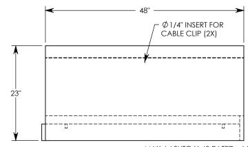
**NOTE 1:** FOR NON-STANDARD LENGTHS THE CHANNEL WILL BE SOLID BOTTOM AND DESIGNATED WITH ITS CORRESPONDING LENGTH MEASUREMENT. IE: HTF2416 32"
