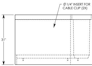
MAX AASHTO H-40 RATED - 64,000 LB. SINGLE AXLE LOAD DEPENDENT ON TRENCH COVER RATING MINIMUM ALLOWABLE SOIL BEARING PRESSURE – H-40: 3,000 PSF; H-20: 3,000 PSF
