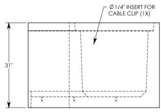
MAX AASHTO H-40 RATED - 64,000 LB. SINGLE AXLE LOAD DEPENDENT ON TRENCH COVER RATING MINIMUM ALLOWABLE SOIL BEARING PRESSURE – H-40: 3,500 PSF; H-20: 3,000 PSF
