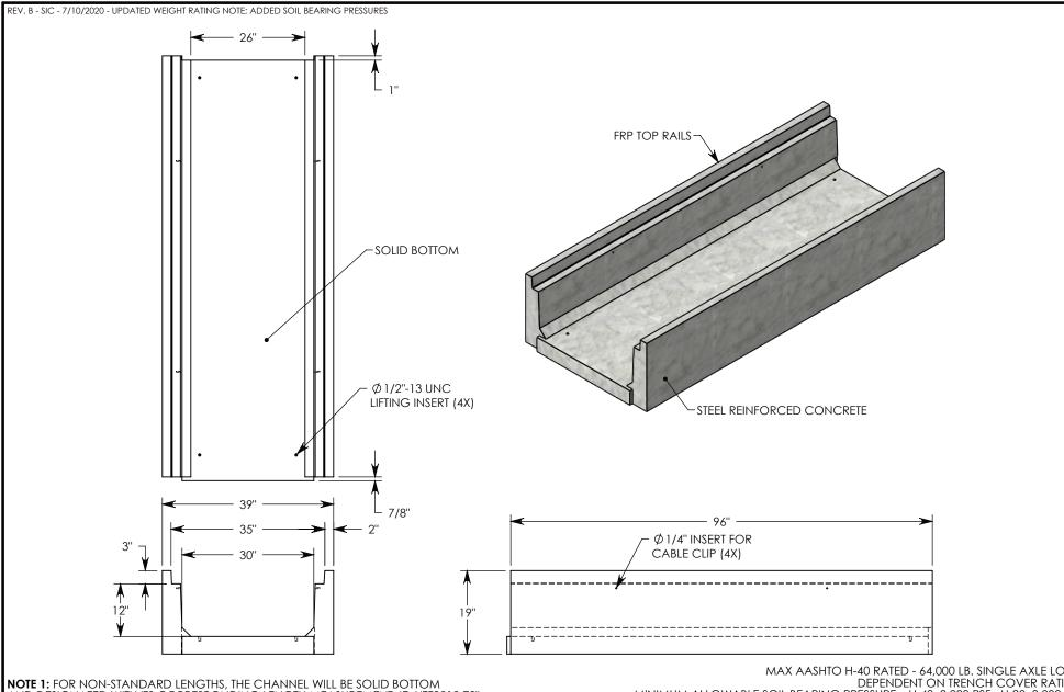
**NOTE 1:** FOR NON-STANDARD LENGTHS, THE CHANNEL WILL BE SOLID BOTTOM AND DESIGNATED WITH ITS CORRESPONDING LENGTH MEASUREMENT. IE: HTF3012 72"
