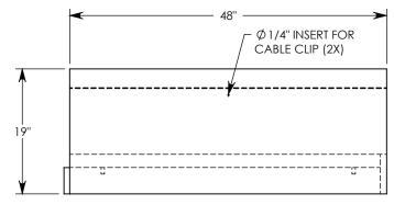
**NOTE 1:** FOR NON-STANDARD LENGTHS THE CHANNEL WILL BE SOLID BOTTOM AND DESIGNATED WITH ITS CORRESPONDING LENGTH MEASUREMENT. IE: HTF3012 32"
