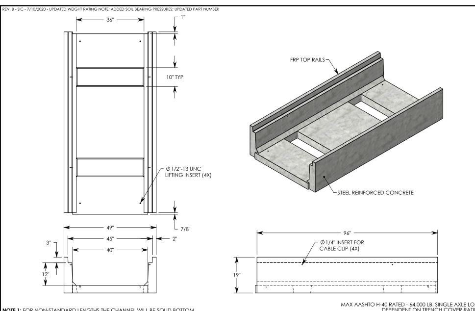
**NOTE 1:** FOR NON-STANDARD LENGTHS THE CHANNEL WILL BE SOLID BOTTOM AND DESIGNATED WITH ITS CORRESPONDING LENGTH MEASUREMENT. IE: HTF4012 32"
