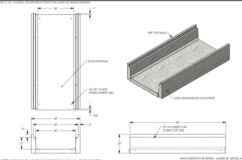
**NOTE 1:** FOR NON-STANDARD LENGTHS THE CHANNEL WILL BE SOLID BOTTOM AND DESIGNATED WITH ITS CORRESPONDING LENGTH MEASUREMENT. IE: HTF4012 72"
