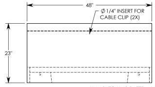
**NOTE 1:** FOR NON-STANDARD LENGTHS THE CHANNEL WILL BE SOLID BOTTOM AND DESIGNATED WITH ITS CORRESPONDING LENGTH MEASUREMENT. IE: HTF4016 32"
