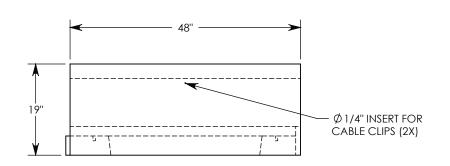
**NOTE 1:** FOR NON-STANDARD LENGTHS THE CHANNEL WILL BE SOLID BOTTOM AND DESIGNATED WITH ITS CORRESPONDING LENGTH MEASUREMENT. IE: LTF4012 36"
