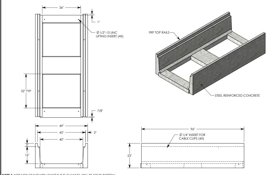
**NOTE 1:** FOR NON-STANDARD LENGTHS THE CHANNEL WILL BE SOLID BOTTOM AND DESIGNATED WITH ITS CORRESPONDING LENGTH MEASUREMENT. IE: LTF4016 36"
