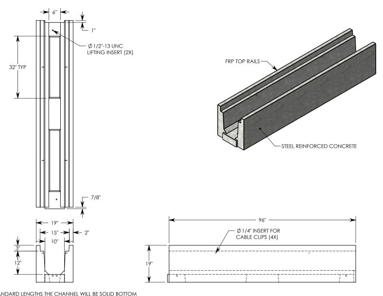
**NOTE 1:** FOR NON-STANDARD LENGTHS THE CHANNEL WILL BE SOLID BOTTOM AND DESIGNATED WITH ITS CORRESPONDING LENGTH MEASUREMENT. IE: LTF1012 36"
