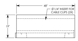
**NOTE 1:** FOR NON-STANDARD LENGTHS THE CHANNEL WILL BE SOLID BOTTOM AND DESIGNATED WITH ITS CORRESPONDING LENGTH MEASUREMENT. IE: LTF1012 36"
