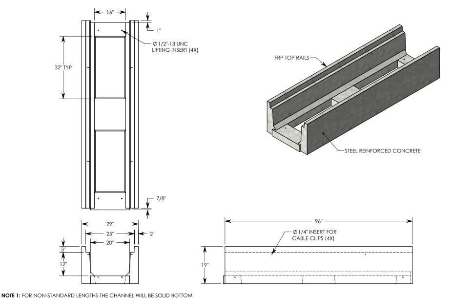
**NOTE 1:** FOR NON-STANDARD LENGTHS THE CHANNEL WILL BE SOLID BOTTOM AND DESIGNATED WITH ITS CORRESPONDING LENGTH MEASUREMENT. IE: LTF2012 36"
