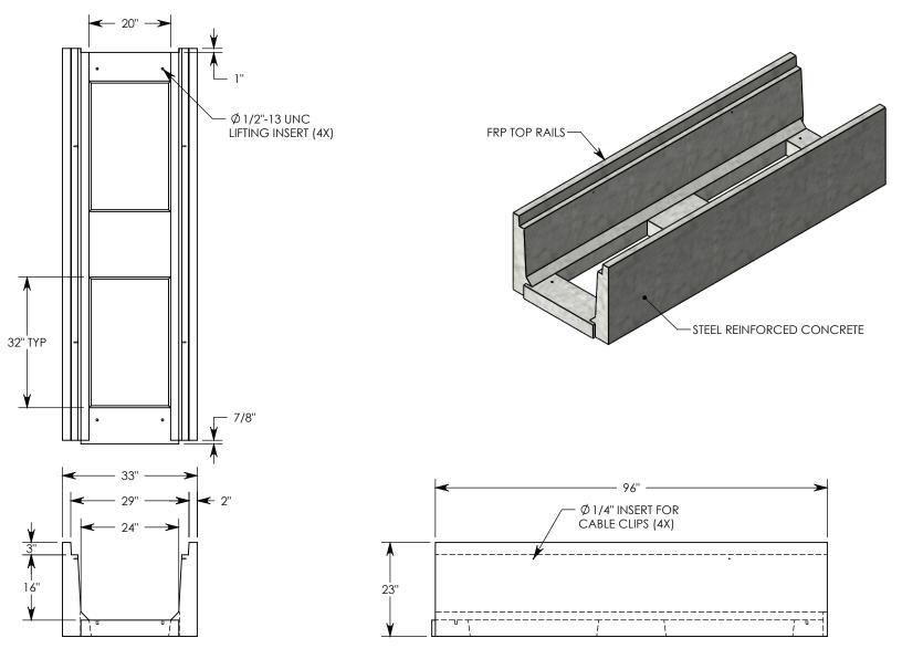
**NOTE 1:** FOR NON-STANDARD LENGTHS THE CHANNEL WILL BE SOLID BOTTOM AND DESIGNATED WITH ITS CORRESPONDING LENGTH MEASUREMENT. IE: LTF2416 36"
