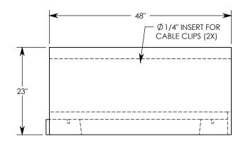
**NOTE 1:** FOR NON-STANDARD LENGTHS THE CHANNEL WILL BE SOLID BOTTOM AND DESIGNATED WITH ITS CORRESPONDING LENGTH MEASUREMENT. IE: LTF2416 36"
