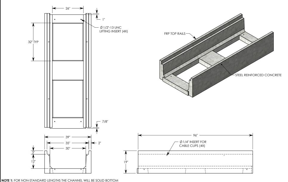
**NOTE 1:** FOR NON-STANDARD LENGTHS THE CHANNEL WILL BE SOLID BOTTOM AND DESIGNATED WITH ITS CORRESPONDING LENGTH MEASUREMENT. IE: LTF3012 36"
