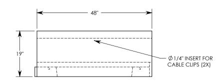
**NOTE 1:** FOR NON-STANDARD LENGTHS THE CHANNEL WILL BE SOLID BOTTOM AND DESIGNATED WITH ITS CORRESPONDING LENGTH MEASUREMENT. IE: LTF3012 36"
