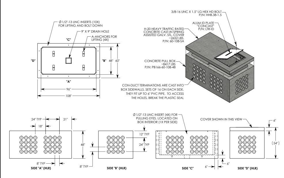
NOTE 1: FOR ADDED SECURITY, PENTA HEAD (P/N: PTA.38-1.5) OR SURELOCK BOLTS (P/N: SL.38-1.25) CAN BE ADDED
