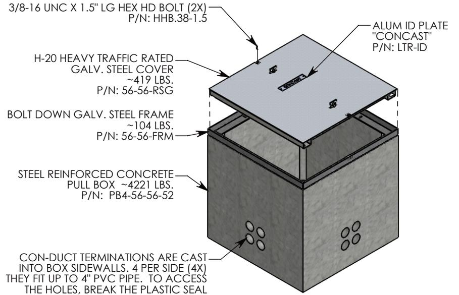
CON-DUCT TERMINATIONS ARE CAST INTO BOX SIDEWALLS. 4 PER SIDE (4X) THEY FIT UP TO 4\"/>
