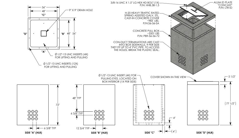
NOTE 1: FOR ADDED SECURITY, PENTA HEAD (P/N: PTA.38-1.5) OR SURELOCK BOLTS (P/N: SL.38-1.5) CAN BE ADDED NOTE 2: FOR PVC SIZES SMALLER THAN 4", USE CONCAST RC41 (REDUCING COUPLER)
