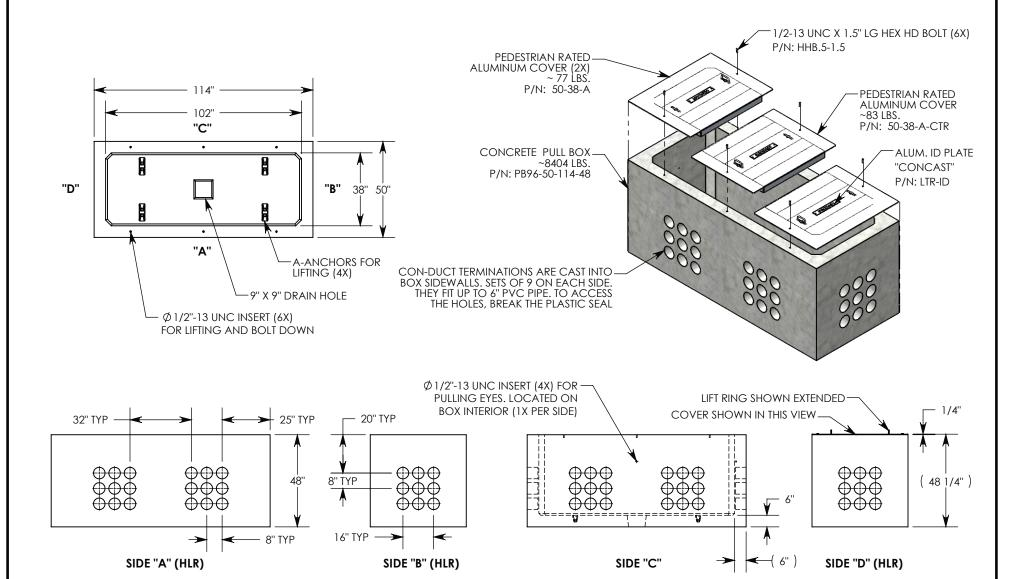
NOTE 1: FOR ADDED SECURITY, PENTA HEAD BOLTS (P/N: PTA.5-1.5) CAN BE ADDED
