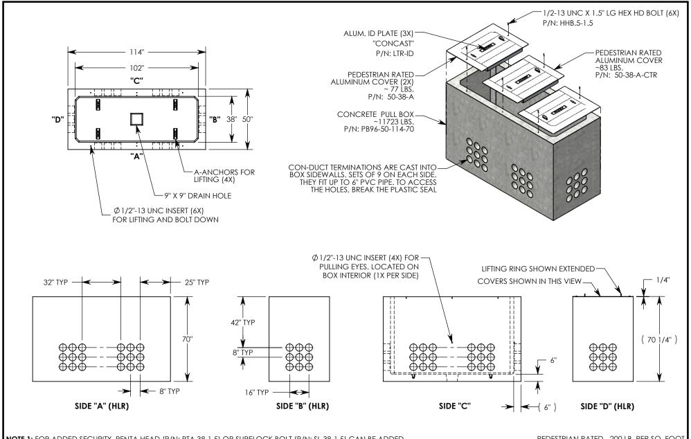
NOTE 1: FOR ADDED SECURITY, PENTA HEAD (P/N: PTA.38-1.5) OR SURELOCK BOLT (P/N: SL.38-1.5) CAN BE ADDED
