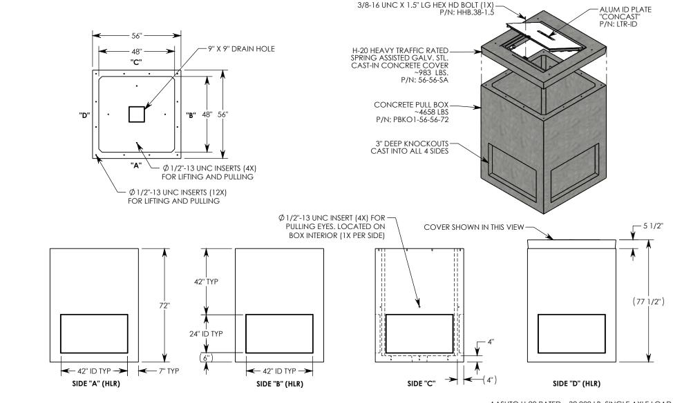
NOTE 1: FOR ADDED SECURITY, PENTA HEAD (P/N: PTA.38-1.5) OR SURELOCK BOLTS (P/N: SL.38-1.5) CAN BE ADDED
