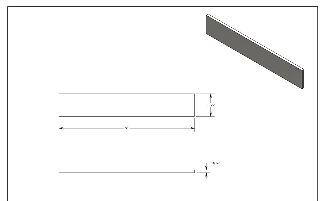
WELD STRAPS ARE TO BE USED WITH EMBEDDED WELD PLATES.
