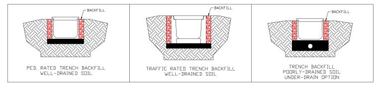
A bed of coarse rock is recommended to bring the yard up to final grade. The final grade must be maintained flush with the top of the road crossing sections. At high frequency traffic areas, the earth should be well compacted. A cement slurry or a concrete apron is also recommended. This will reduce impact loading and possible chipping and cracking on the edges of channels.
