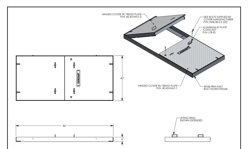
NOTE 1: FOR ADDED SECURITY, PENTA HEAD (P/N: PTA.38-2.5) OR SURELOCK BOLTS (P/N: SL.38-2.5) CAN BE ADDED
