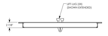
NOTE 1: FOR ADDED SECURITY, PENTA HEAD (P/N: PTA.38-1.5) OR SURELOCK BOLTS (P/N: SL.38-1.25) CAN BE ADDED NOTE 2: TREAD ON DIAMOND PLATE ADDS 1/8" TO OVERALL HEIGHT
