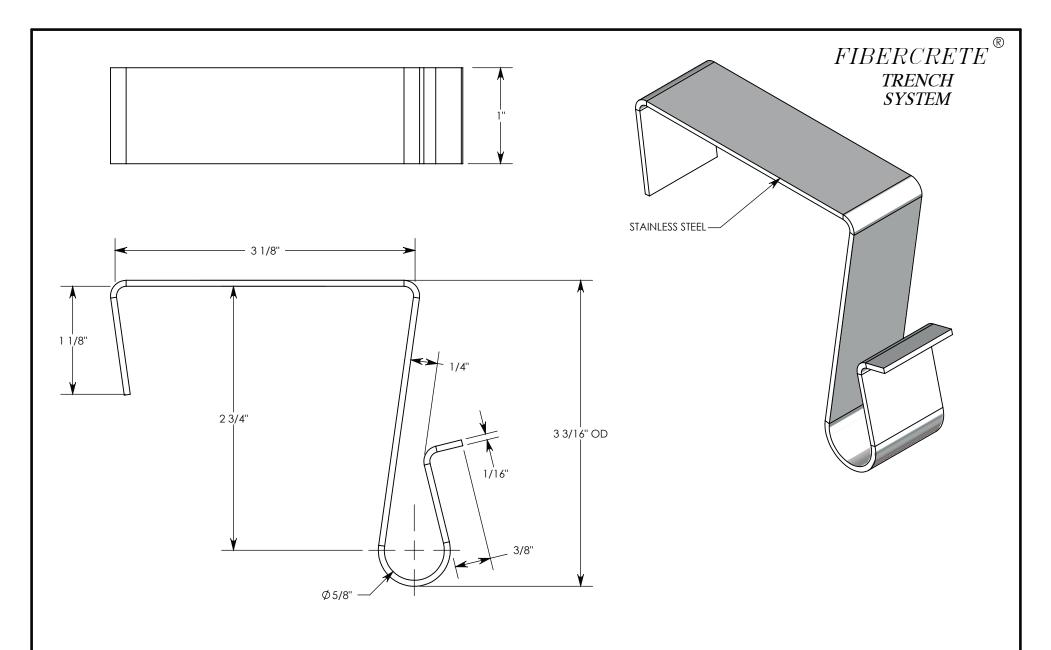
CHANNELS ARE NOTCHED FOR GROUND CABLE CLIPS.
