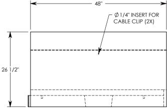
MAX AASHTO H-40 RATED - 64,000 LB. SINGLE AXLE LOAD DEPENDENT ON TRENCH COVER RATING MINIMUM ALLOWABLE SOIL BEARING PRESSURE – H-40: 3,500 PSF; H-20: 3,000 PSF
