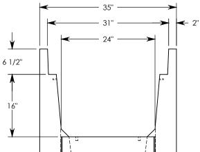
**NOTE 1:** FOR NON-STANDARD LENGTHS THE CHANNEL WILL BE SOLID BOTTOM AND DESIGNATED WITH ITS CORRESPONDING LENGTH MEASUREMENT. IE: 802416HT 32"
