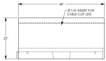
**NOTE 1:** FOR NON-STANDARD LENGTHS THE CHANNEL WILL BE SOLID BOTTOM AND DESIGNATED WITH ITS CORRESPONDING LENGTH MEASUREMENT. IE: 802416HT3 32"
