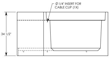
AASHTO H-20 RATED - 32,000 LB. SINGLE AXLE LOAD MINIMUM ALLOWABLE SOIL BEARING PRESSURE – 3,000 PSF
