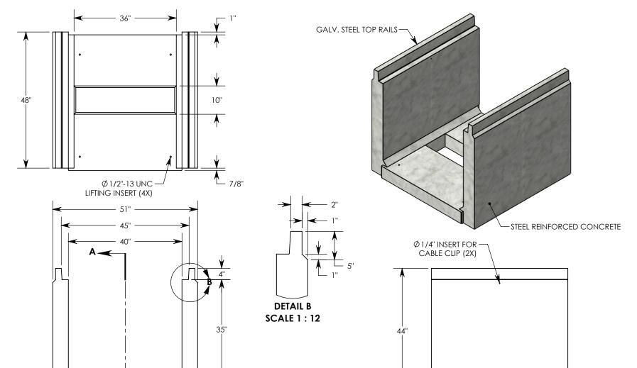
NOTE 1: FOR NON-STANDARD LENGTHS, THE CHANNEL WILL BE SOLID BOTTOM AND DESIGNATED WITH ITS CORRESPONDING LENGTH MEASUREMENT. IE: 804036HT4 32"
