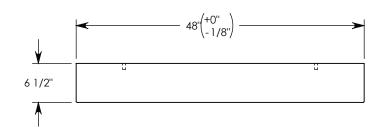
**NOTE 1:** FOR NON-STANDARD LENGTHS, THE PART NUMBER WILL CORRESPOND TO IT'S MEASURED LENGTH. IE: 8041HT 18"
